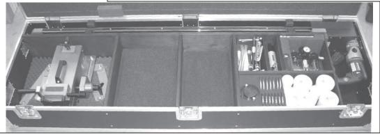
Pneumatically driven machines also require the accessory pneumatic motor maintenance kit
