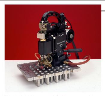
The Model 6 is a rugged, field-proven weld head for high-production welding of tube-to- tubesheet using the GTAW process. The Model 6 has exceptionally fast mount and dismount times for ease of operation and productivity. The torch is positioned on the tube to be welded by a pneumatically operated locating fixture. With the touch of a button, the locating fixture precisely locates itself over the tube to be welded.
