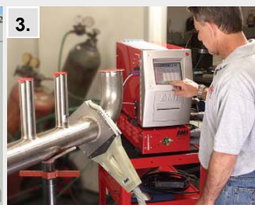
Weld Schedule Modification Values of Amps, pulse rate, travel speed, and wire feed rate may be instantly raised or lowered at the touch of a button.
