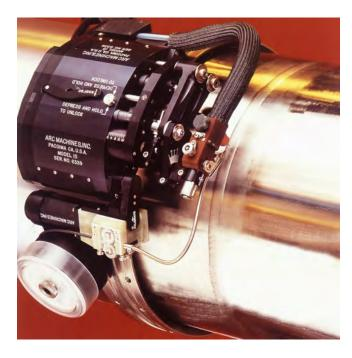
The Model 15 is a rugged, precision weld head with low radial and axial clearance for GTAW welding of all pipe sizes from 3 inch (76 mm) OD pipe up to an unlimited size, including flat plate. It is primarily designed for field use where exceptional weld quality and consistent results are required.
