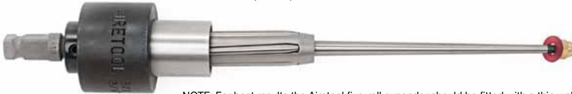
NOTE: For best results the Airetool five-roll expander should be fitted with a thin wall thrust collar when being used to roll tubing with 20 BWG .035" (0.9 mm).
