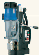
MAB 825, MAB 825 V & MAB 845 p. 22 Capacity: \varnothing 4" cutter; \varnothing 1-1/4" twist drill; \varnothing 1-1/8" tapping Auto feed (MAB 825 V) Swivel base (MAB 845) Reversible, 4-gear motor
